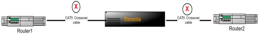
**Figure 10:** *Inline deployment scenario, router to router server*
