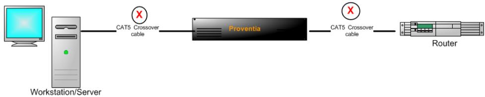
**Figure 7:** *Inline deployment scenario, workstation server to router*
