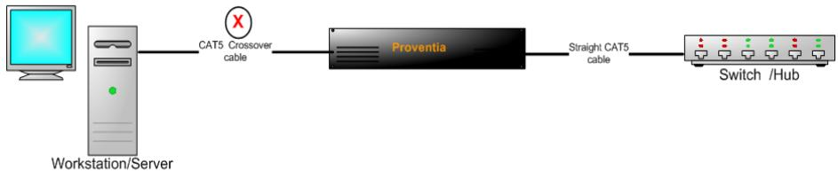
**Figure 8:** *Inline deployment scenario, workstation server to switch/hub*
